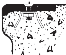
Type 101 with wing type anchors in poured concrete stair.
