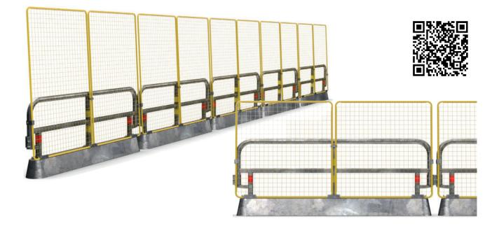
GC Fence can also be mounted on a footplate like traditional construction fencing. It's then available in different heights, and it can be set up easily and without heavy lifting (max. 20 kg / 44 lbs): short net 1,400 mm (4' 7"), long net 2,100 mm (6' 11").
