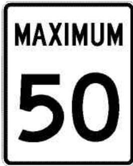
**Location data:** Required sign is 50 km/h, size is 600 mm x 750 mm.
