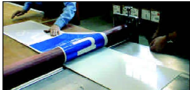
Figure 4.24 – Positioning of Transfer Tape and Transparent Sheeting (with backing) on Reflective White Background Sheeting on Substrate
