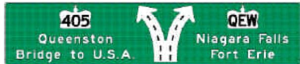
**Location data:** Posted speed is 100 km/h; rural freeway (QEW) (three lanes each direction); overhead sign; good vertical and horizontal alignment. Sign to depict diagrammatically a three-lane roadway splitting into two two-lane roadways, with an either/or lane.
