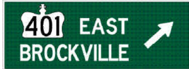
**Location data:** Posted speed is 70 km/h; municipal two-lane road (one lane each direction); no space constraints; ground-mounted sign; good vertical and horizontal alignment.
