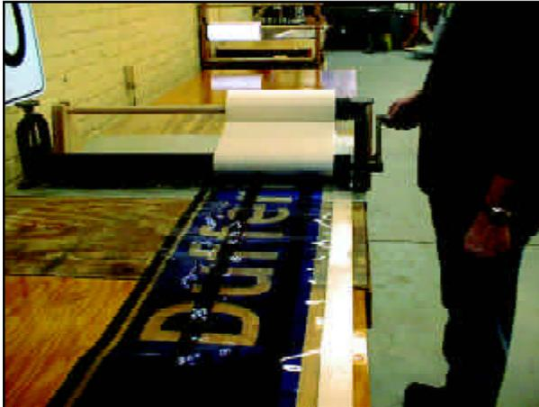
Figure 4.26 – Stripping of Backing from Reverse-cut Transparent Sheeting (second half)
