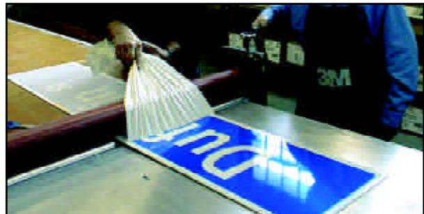
Figure 4.25 – Stripping of Backing from Reverse-cut Transparent Sheeting (first half)
